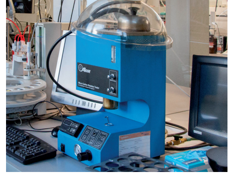
Now used for fuel analysis: Micro Conradson test apparatus
