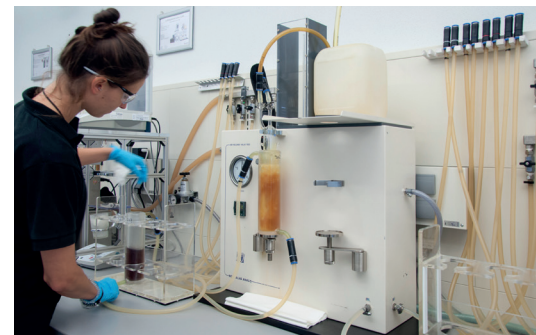
Determining the LAV in the OELCHECK laboratory using the Analis P 688 testing standard lab
