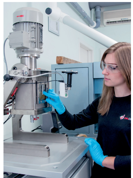
Flender foam test – a reading is taken of the increase in oil volume
