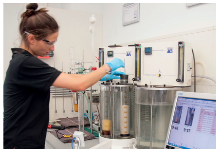
Determining the foaming tendency in the OELCHECK laboratory using the Analis P 643 testing standard lab
