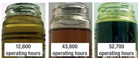
Discolouration of the synthetic gear oil
