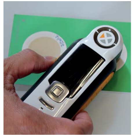
MPC-Test – Filter evaluation with a colorimeter.
