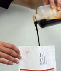
❶ We put it to the test and filled 200 ml of oil directly into the delivery pouch instead of a sample container.
