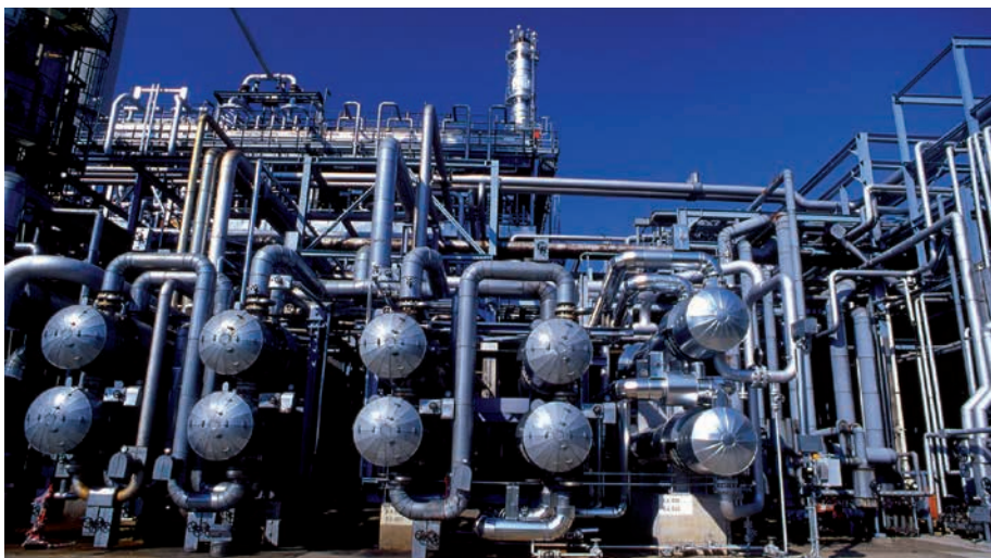
CHD heat exchangers – the product fed into the system is heated to initiate the chemical reaction with the catalyst.
