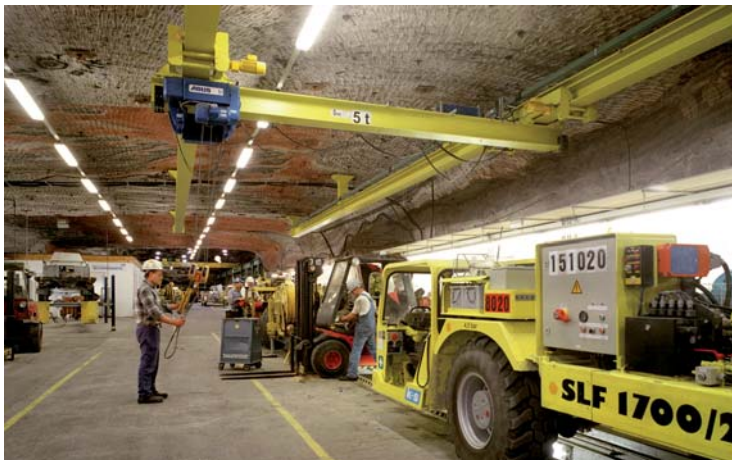
In the 20,000 m 2 workshop, the devices are serviced and repaired underground.
