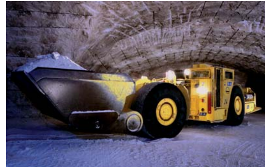
The crude salt, loosened by blasting, is transported to the crushers using wheel loaders. K+S KALI GmbH produces 8 million tonnes of potash fertilizer in Germany per annum.
