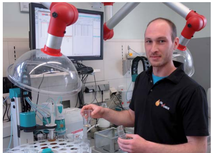
Measuring the Neutralisation Number for refrigerating machine oils in the OELCHECK laboratory
