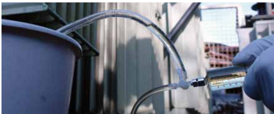
Sampling in a glass syringe, on the left in the figure: Bucket as a flushing container
