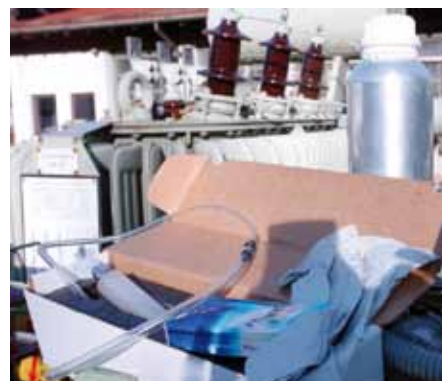
Analytical set for transformer oils: Shipping carton with 20 ml glass syringe, sampling tube, protective gloves, paper towels, test data sheet and optional 1 litre aluminium bottle
