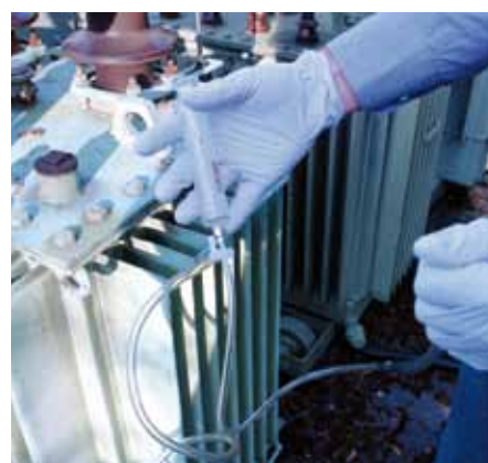
Glass syringe prepared for sampling, including a 3-way stopcock and sampling tubes
