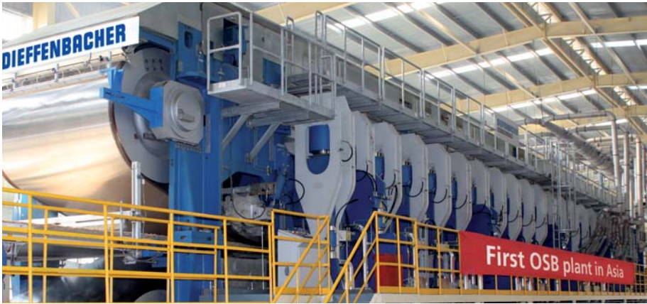
CPS endless presses for the manufacturing of chipboard
